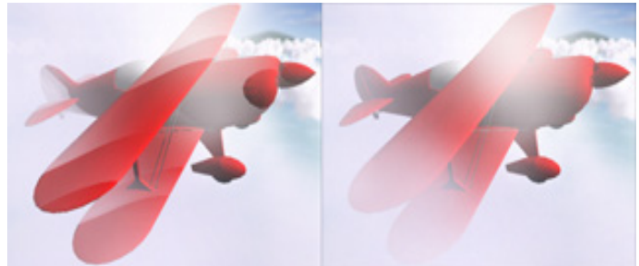
Figure 12 An airplane in the clouds. On the left, particles are directly rendered into the scene. Artifacts of their intersection with the plane are visible. On the right, the airplane is rendered between impostor layers, and no artifacts are visible.
