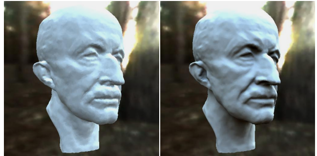
Figure 1: Precomputed, unshadowed irradiance from [34] (left) vs. our precomputed transfer (right). The right model can be rendered at 129Hz with self-shadowing and self-interreflection in any lighting environment.
