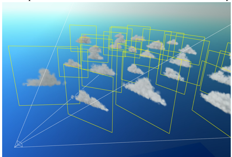
Figure 10: Impostors, shown outlined in this image, are textured polygons oriented toward the viewer.
