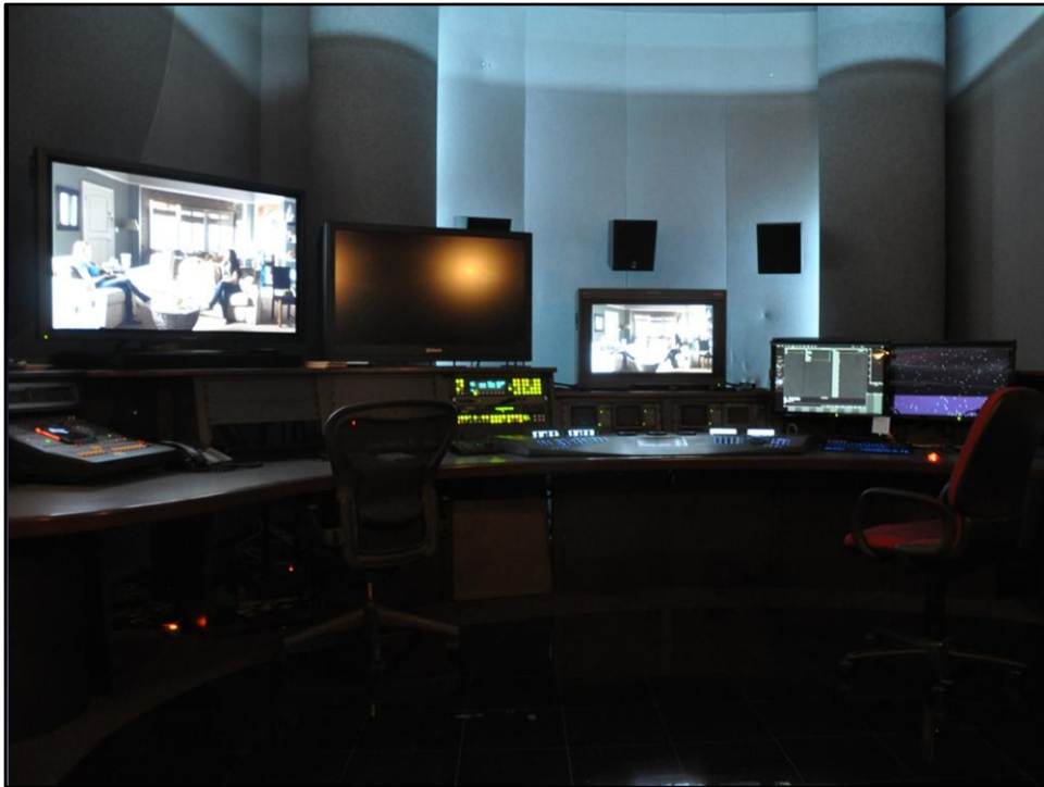
This picture shows a non-projection grading environs, with a 32" CRT reference and a 50" plasma display that matches to a fairly high degree.
